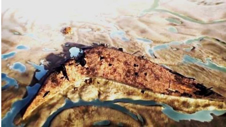
The wreck of Fuso as faithfully rendered in capture from Drain the Oceans episode " Mega Wrecks " Season 2-Episode 8 . It shows at a glance how the battleship's hull still essentially forms one single piece but upside down and boomerang shaped. Notice also the large defect/gash in the port quarter just forward of the propellers and how the rudders are turned. Part of the pagoda foremast is just above and nearly due north of the buckle point.(Drain the Oceans)
