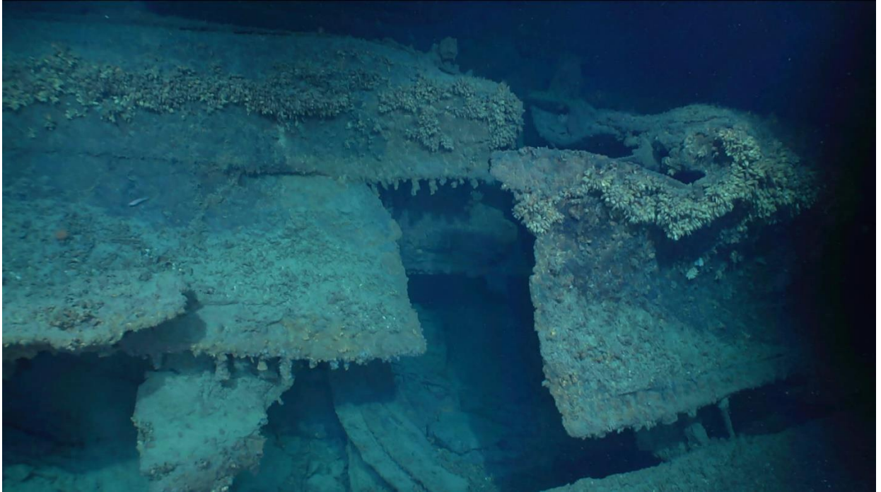
This is Fuso's centerline keel at frame 260 looking from the starboard side and it shows Daly's torpedo hit at the same location from port snapped the keel in half. (Photograph provided by Lone Wolf Media.)
